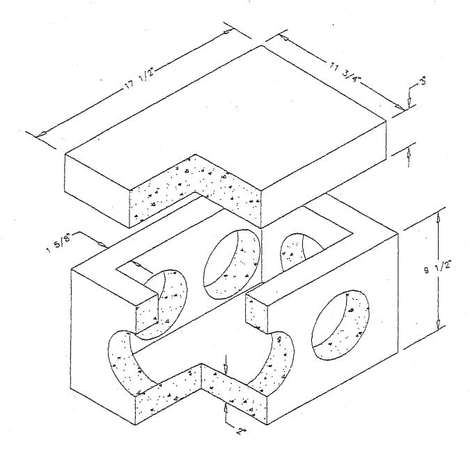
Distribution Box is Reinforced with #9 wire Crisscrossed on bottom that continues up the sides, corners, and around the top.
